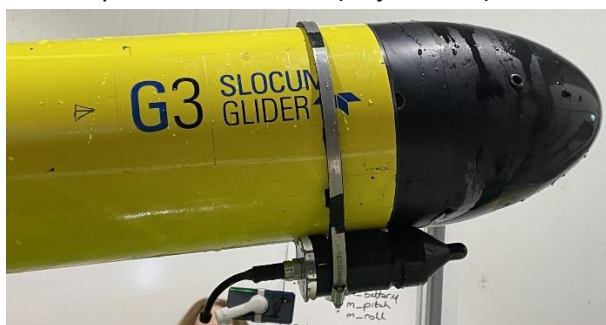
Figure 1: The soundtrap pointing forward and attached under the hull of the G3 Slocum glider.
