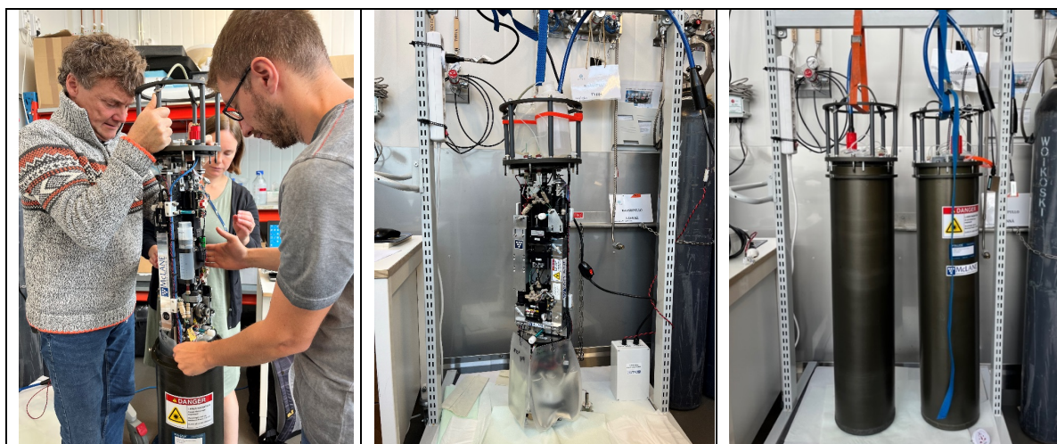
Figure 1. Setting up the IGB-IFCB (left, Jens Nejtgaard, Kaisa Kraft, Christian Dilewski); Naked hung up IGB-IFCB filled with fluids and ready to measure (mid); IGB-IFCB (135) and SYKE-IFCB (114) ready be installed in the AQUABOX (right); (Photos: Stella A. Berger, IGB).
