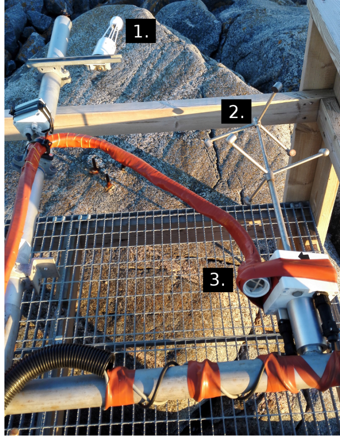
Figure 11: The top of the flux tower. From top to bottom: LI-7500 (Licor) open-path gas analyzer (1), uSonic-3 (Metek) anemometer (2) and the inlet for closed-path analyzers (3).
