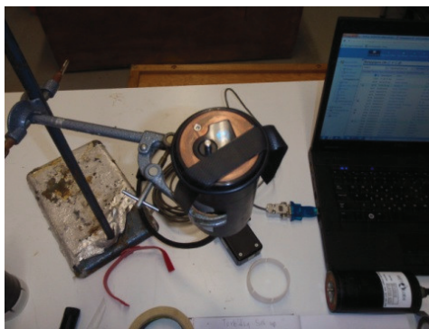
The turbidity calibration set-up.
