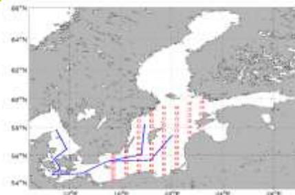
The OSSE experiments in the Baltic Sea assimilate the T/S profiles from XBT and moored buoy.
