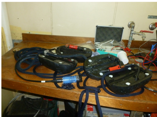
Fig. 2: Photo of the two SQUID and optode. The Squid is made of 2 parts, one with the battery and one with the data logger on which the oxygen optode is connected.
