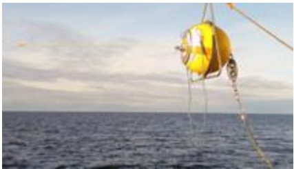
Wave buoys Wave height and direction Temperature
