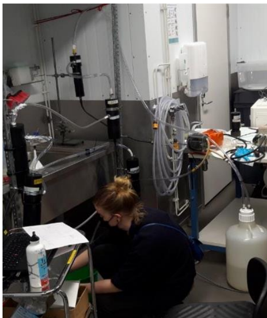
Figure GoF-PSS#1: Left: Calibration of GoF-PSS field fluorometers ongoing. Right, up: Comparison of FerryBox temperature sensor readings with reference sensor. Right, bottom: PSS-GoF CDOM fluorescence sensor responses prior and after joint calibration.
