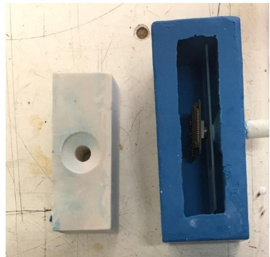
**Figure 10.** Silicon rubber mould for casting the JELAB2 camera and glass.
