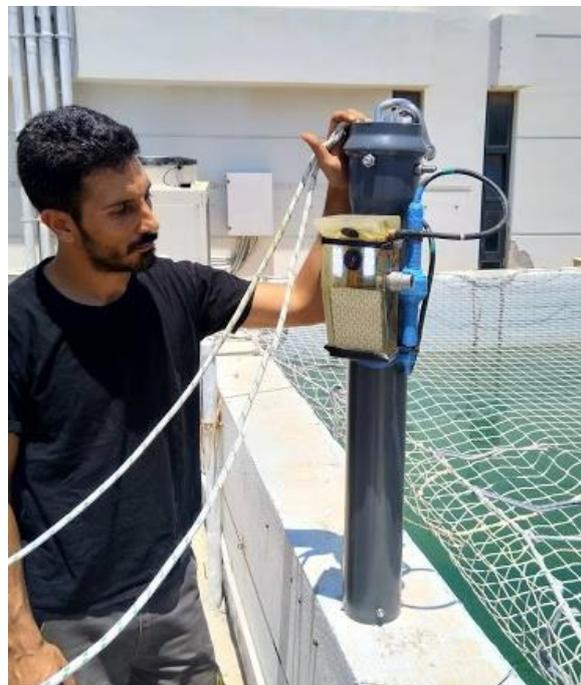
**Figure 16.** The JELAB2 test configuration with battery pack and ballast module.
