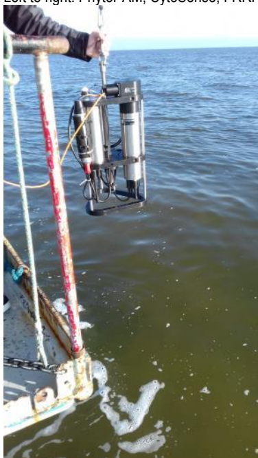
FRRF profiler (two FastOcean Chelsea sensors integrated on an APD system) plus an independent hyperspectral radiometer TRIOS (GmbH) on the "Côte de la Manche" ship.
