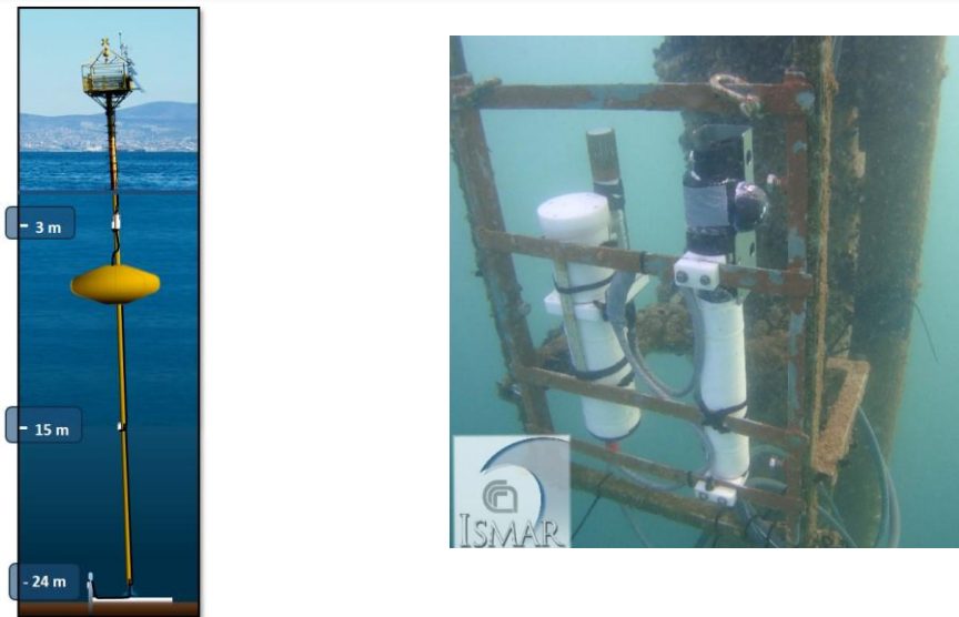
Figure 3.3.5. Scheme of the PALOMA elastic beacon hosting the Contros sensor (left), the sensor installed at 3 m depth (instrument on the left), near a multiparametric CTD probe (right).
