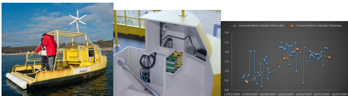
Figure 3.1.4. Molit Buoy, Model of two CHEMINIs inside Molit silicates concentrations in \mu\text{mol/l} during the 2009 deployment in the Vilaine Bay.
