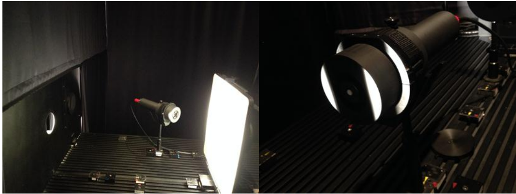
Figure 3.2.12. Example of the optical table used for irradiance sensor calibration.
