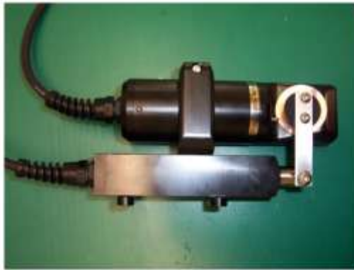
D-Opto dissolved oxygen sensor with Shutter fitted
