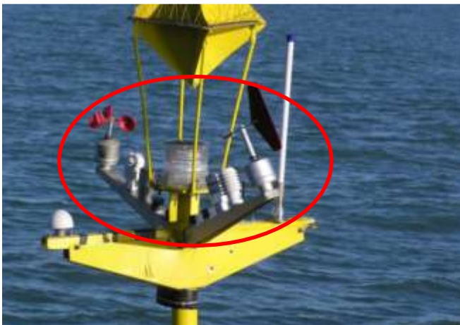
S1 Buoy: Damage to the meteorological mast
