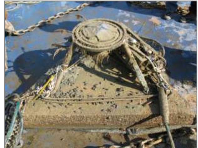
S1 Buoy: ADCP Sensor after one year on the sea bottom
