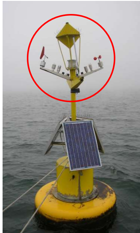
E1 Buoy: Damage to the meteorological mast
