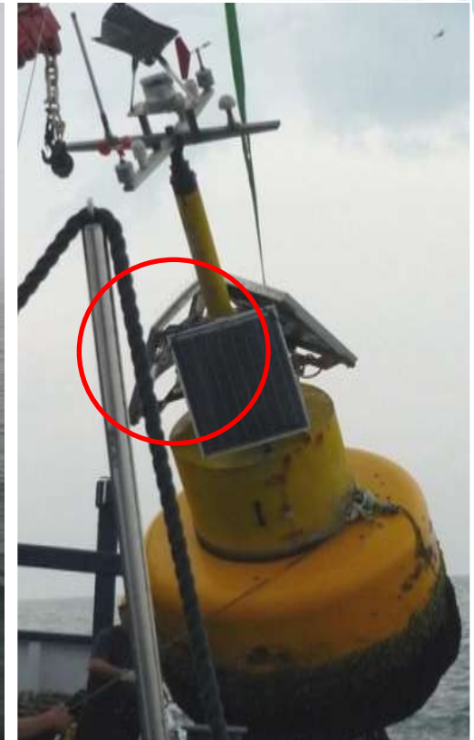
E1 Buoy: Problems to solar panels (breakage or theft)
