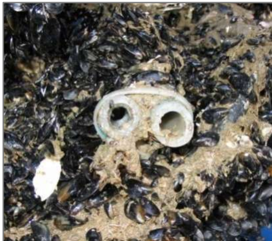
Particular Water suction pipe of E1 CTD SBE 37 after one year at sea
