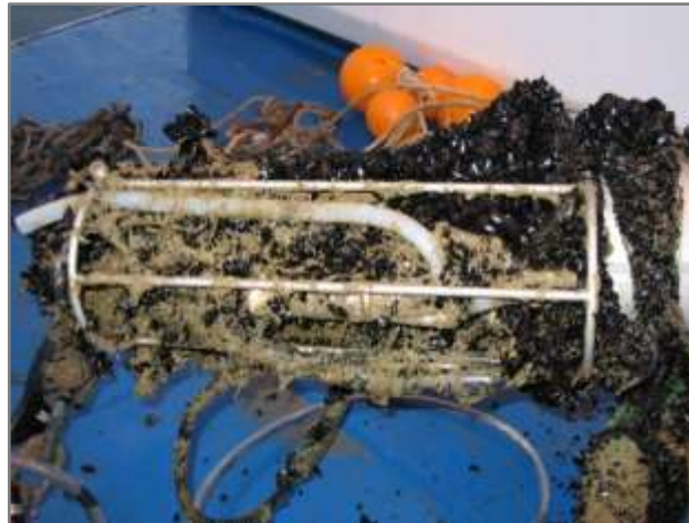
E1 Buoy 1° Level after one year at sea
