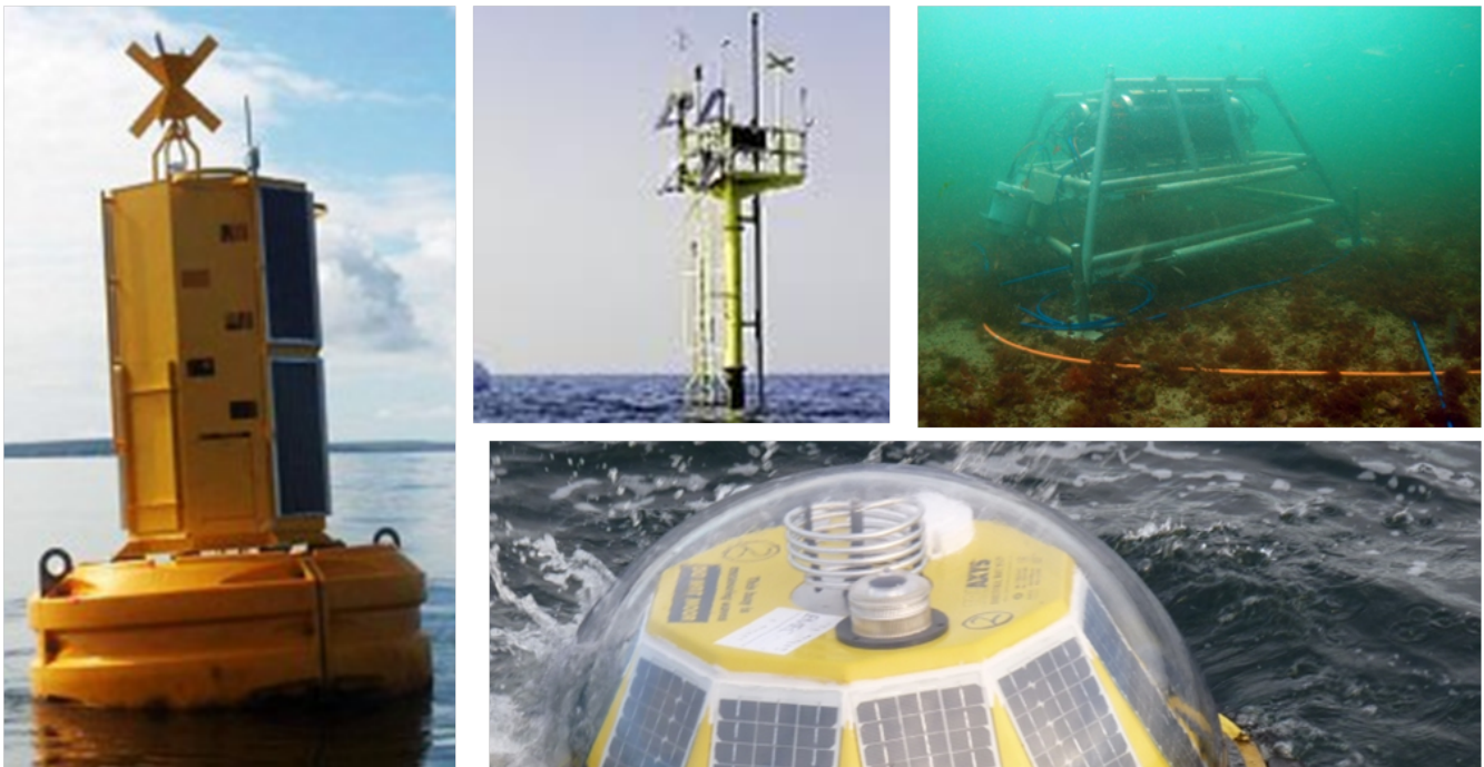
Figure 1: Types of fixed platform observing systems in use in Europe (left panel) surface mooring at SmartBay site, Galway, Ireland (upper mid) Observation tower in the COSYNA network, German Bight, Germany (upper right) underwater node of COYNA, Helgoland, Germany (lower) Wave rider buoy, Cefas Wavenet, UK.
