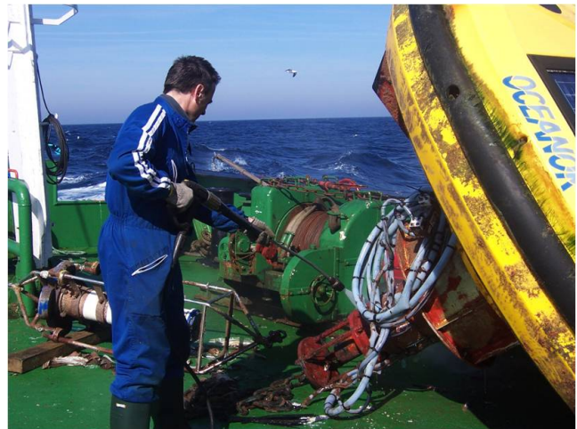
Figure 34: Cleaning biofouling from a Euskalmet/AZTI buoy.
