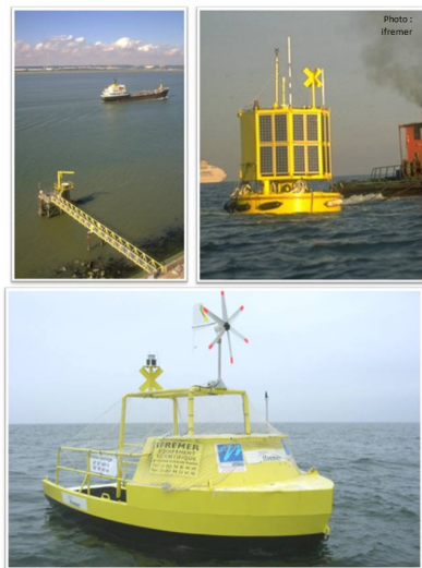
Figure 19: Ifremer fixed platforms showing different designs and methods of power supply (top left) cabled platform at Brest (b) solar powered mooring off the Seine estuary (c) wind powered MOLIT mooring off the Vilaine estuary. (Photos of L. Delauney (IFREMER RTD)).
