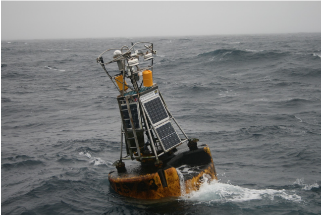
Figure 12: Surface superstructure of the PAP mooring
