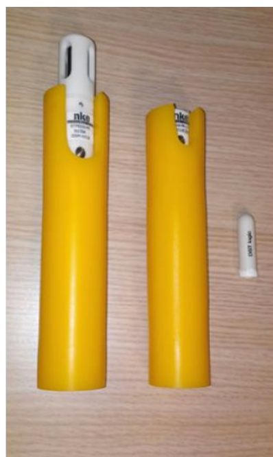
Figure 5 Example of StarOddi sensor (right) and NKE SP2T-R (center), NKE SP2T-R (left) with the protection provided by the manufacturer
