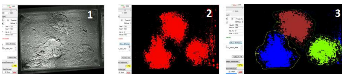
Figure 10 Example of use of AviExplore Fixed Module for the identification of regions with high activity. 1) Gray-scale image, 2) Result of the overall addition of moved pixels, 3) Identification of three regions
