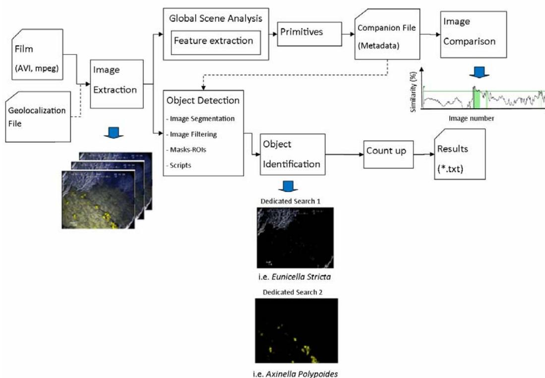
Figure 14. Flowchart of main steps in the analysis of mobile-sourced videos with some examples after processing.
