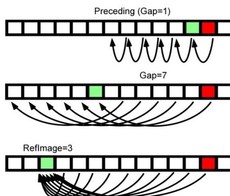
Figure 17. Schematic of different image subtraction modes
