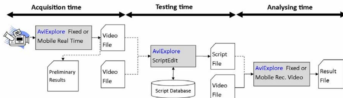
Figure 9. Example of interactions between different modules and modes of AviExplore.
