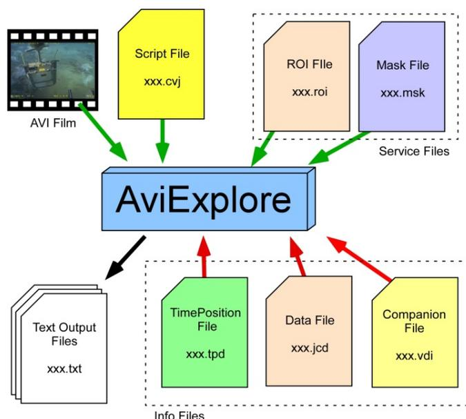
Figure 11. Summary of external companion files related to AviExplore. Green arrows refer to files that need to be loaded by the user. Red arrows refer to file automatically loaded by the software if they exist.
