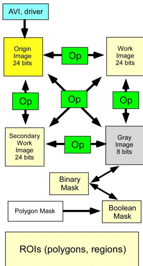
Figure 10. Flowchart of the internal structure of AviExplore. Origin, Work and Secondary Work are 24 bit Bitmaps for color pictures and video frames. The Gray image is a 8 bit image which has connexions with a 8 bit buffer (Mask) used to store intermediate measures. ROIs are polygonal structures saved in external files which can be loaded upon demand
