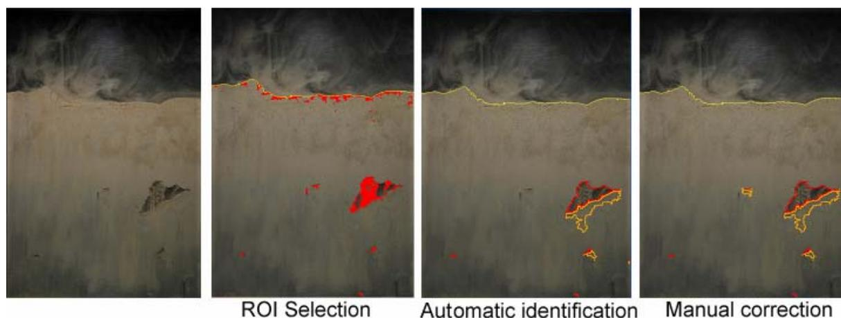
**Figure 4. Example of image processing at each intermediate step constitutive of the analysis of biogenic structures**
