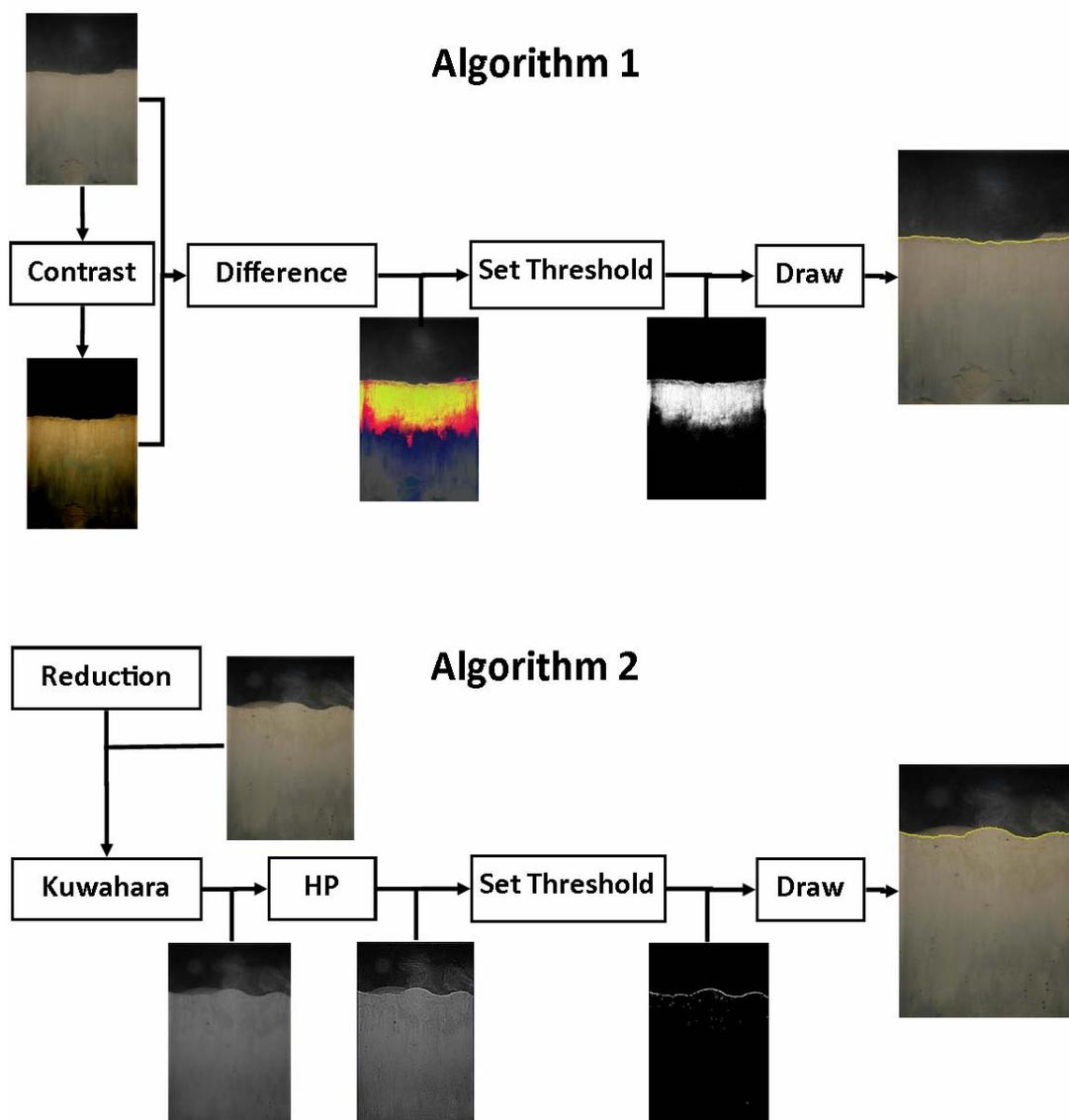
Figure 3. Flowcharts of the 2 algorithms used to draw the sediment-water interface. Examples of image processing at each intermediate step are provided for both algorithms
