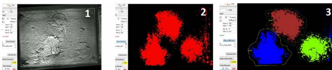
Figure 28. Example of use of AviExplore Fixed Module for the identification of regions with high activity. 1) Gray-scale image, 2) Result of the overall addition of moved pixels, 3) Identification of three regions
