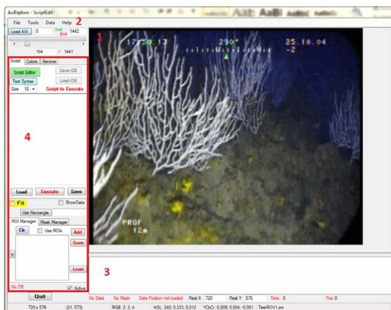
**Figure 12. AviExplore Graphic user interface. Common structures: 1) video display window, 2) strip menu and 3) video time Scrollbar. The red rectangle (4) differs between modules**
