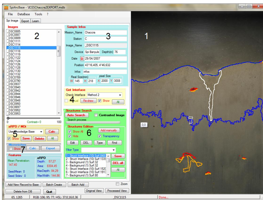
Figure 1. SpiArcBase: Main window. (1) Selected image with overlays of the computed sediment-water interface (in blue), the aRPD (in blue) and biogenic structures (“oxic voids” in red, “associated with oxic voids” in orange and “feeding structure” in white), (2) List of images in the current database, (3) Meta-information related to the acquisition of the selected image, (4) Sediment-water interface drawing/computation, (5) aRPD drawing/computation, (6) Biogenic structure computation and list
