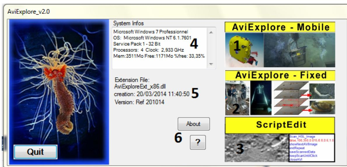
**Figure 8. AviExplore: Starting window.** (1) access to the module related to videos coming from mobile vehicles, (2) access to the module related to videos coming from fixed platforms, (3) access to the module for editing scripts, (4) summary of system characteristics, (5) extension file for evolutive versions of AviExplore and (6) software manual and information
