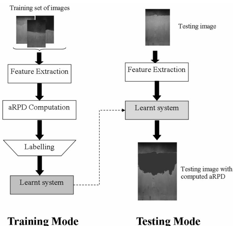
**Figure 5. Machine learnt structure for the computation of the aRPD. A learnt system is built during the training mode and then used during the testing mode.**
