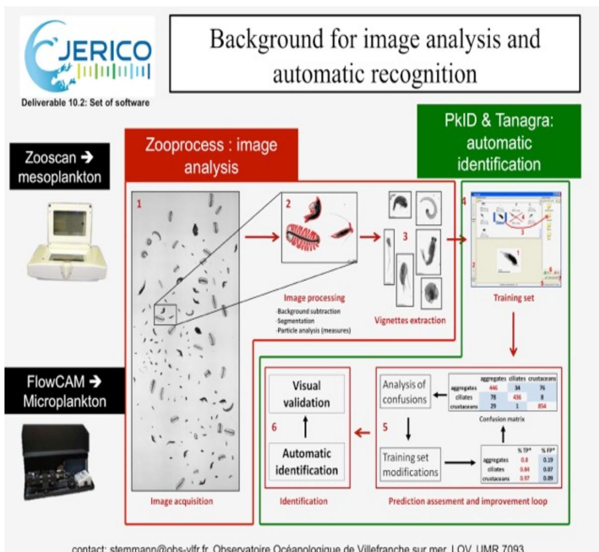
Figure 21 *Flow Diagram illustrating Steps 1 to 6 how the Zooprocess image analysis and automatic recognition software identifies Zooplankton.*
