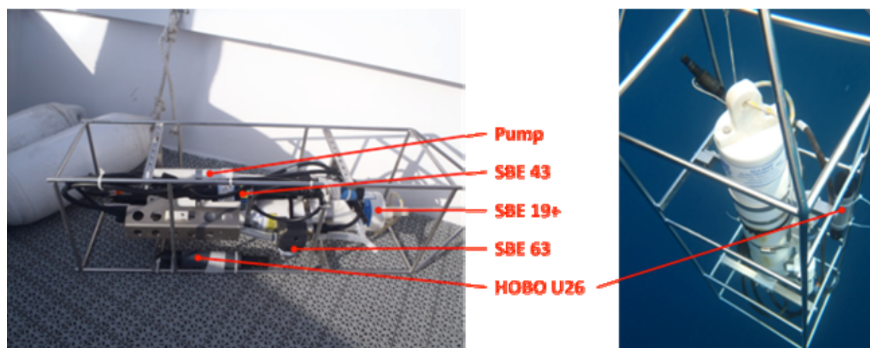
Figure 4: Autonomous CTD/DO used for JERICO inter-comparison exercise (SBE 19+/ SBE 43/ SBE 63/ HOBO U26)
