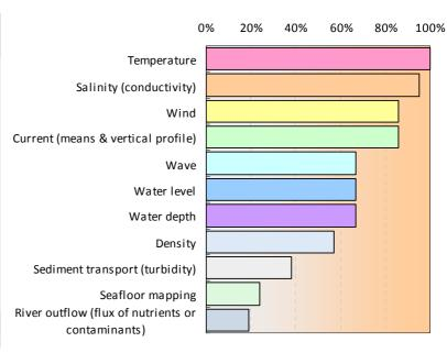
Temperature and salinity were the most cited by the JERICO community with regards to physical parameters. Wind and current were also largely cited for this question. In the 'other' section were also specified parameters like:
