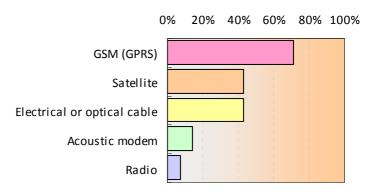
The survey again shows that GSM is the most common used technology to transfer data from the sensors. In the 'other' section were specified technologies like:
