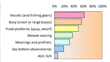
As for the other sensors, the most common platforms are vessels, buoys and fixed platforms. In the 'other' section were also cited platforms such as:
