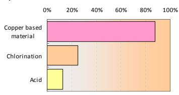
Copper based materials are the most cited method to prevent bio-fouling. Other methods mentioned were:
