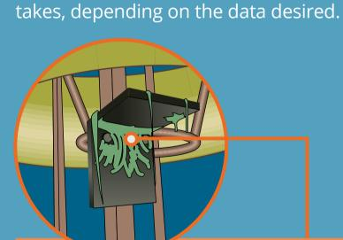
Settling plates can be added to the underside of the SmartBuoy to determine which invasive non-native species are present.
