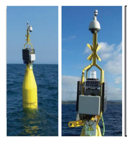
IP Camera: 704x576 pixels; 25 fps; 10x Optical Zoom Solar panels: 4 x 20W Weather station: Position, velocity and GPS time Speed and wind direction Pressure and temperature magnetic compass 3-axis accelerometer for Pitch and Roll angles Buoy signalling light, self-powered: High efficiency yellow LED light Reach 3 nautical miles Junction box **Electronic Control 3G Modem Communication Battery Box** Battery: 12v & 65Ah Solar charge controller: 6A
