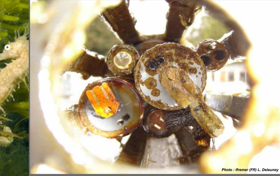
Materials and shape shoud be choosed very carefully in order to reduce fouling attachement.
