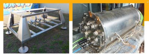
Deploy a new video camera with a custom housing and a wipper to avoid biofouling
