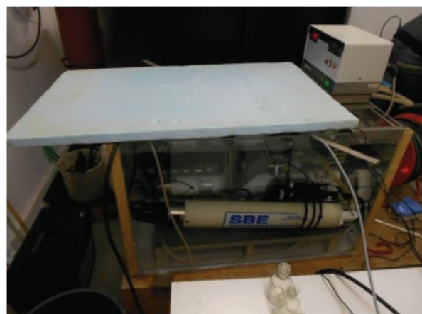
The two SBE43 installed on the SBE16 ready for the oxygen calibration and the experimental set-up.
