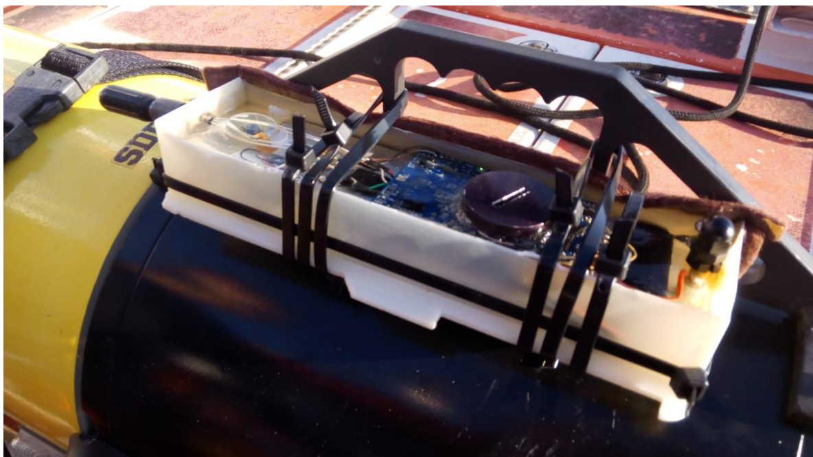
Figure 2- The acoustic datalogger (BCB, Loggerhead Instrument) was turned on following the selected schedule and attached to the SOCIB glider SDEEP04
