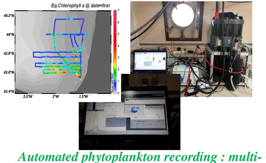
spectral fluorometer (continuous and profiling) & automated flow cytometer + imaging in flow
