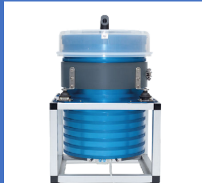
The CytoSense flow cytometer (Cytobuoy©)
