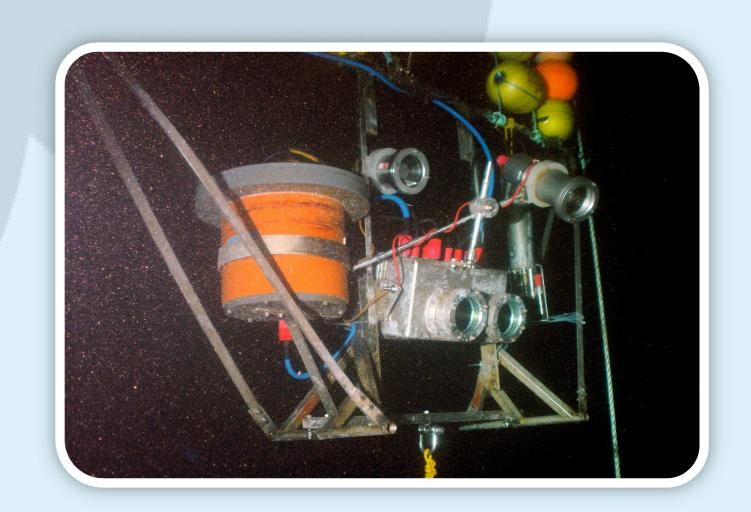
The seabed cabled observatory **EMSO-Molène** was deployed off shore 2 km north of Molène, in the marine protected area "Iroise Marine Park". It is an EMSO testing site at depth 18 meters, dedicated to sensors and equipment in-situ and long-term qualification.
