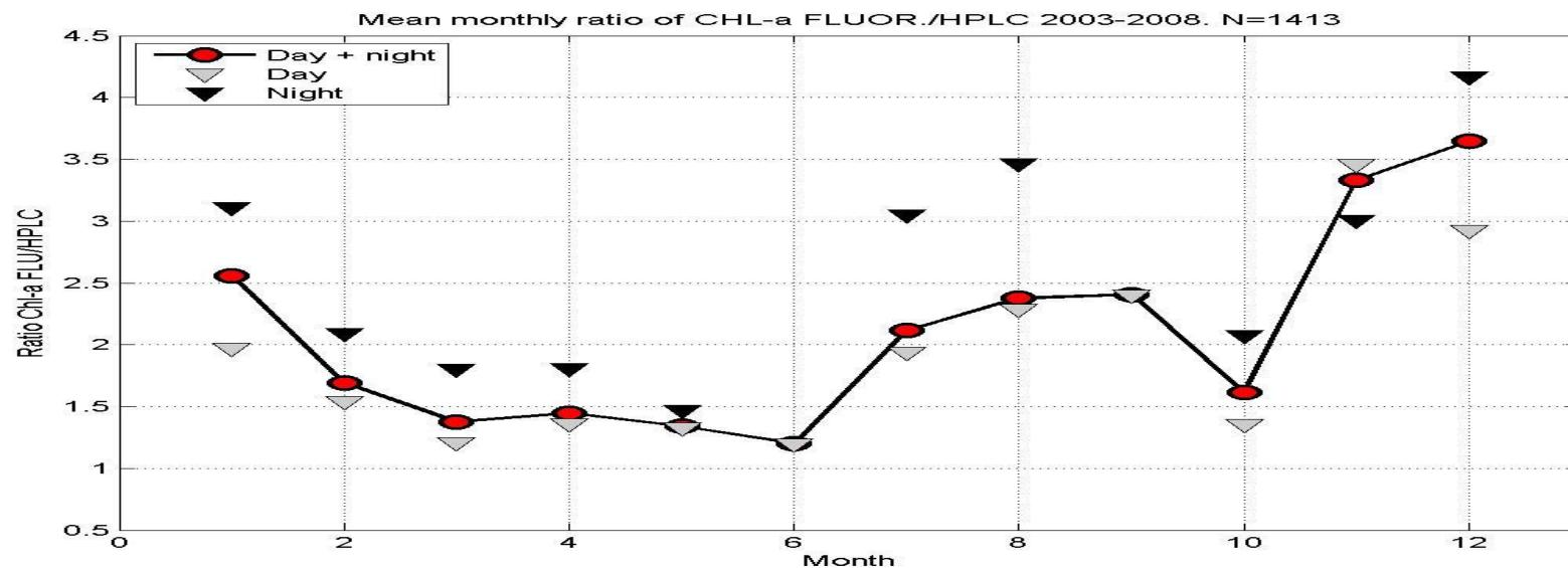
Yearly calibration of the Chl-a fluorescense using all the Chl-a\_hplc water samples
