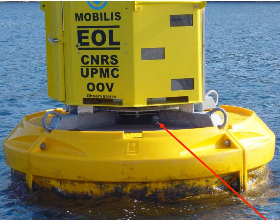
Wave absorber on EOL buoy
