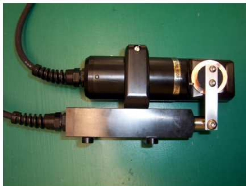
D-Opto dissolved oxygen sensor with Shutter fitted
