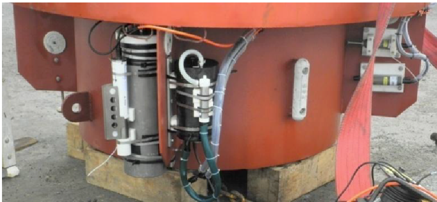
Sensor deployed in 2011 on ESTOC site, including pCO 2 from Pro-Oceanus
