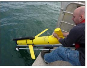
OMG includes Seabird CTD and retro-fitted microstructure (512Hz shear, temperature, conductivity +?)
