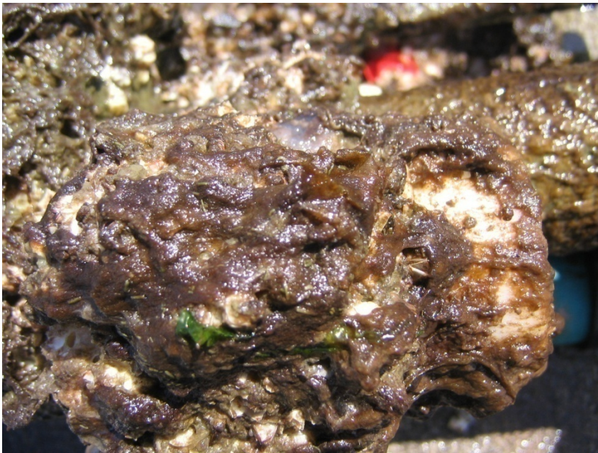
External fouling on instrument does Not impair interior
