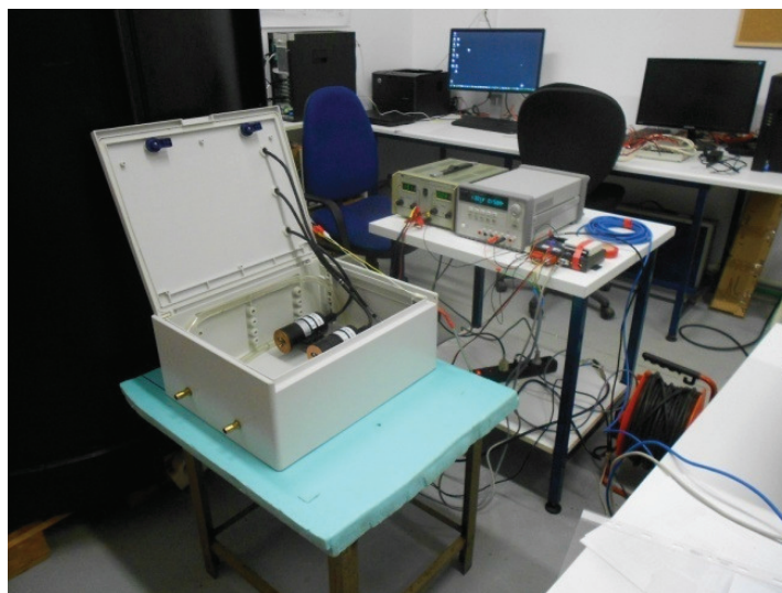
Figure 3. The experimental set-up prepared to perform the fluorescence test. On the foreground is the chamber with the sensors inside. In the background, on the table, the power supplies, the analogue acquisition board and the serial device driver are installed.
