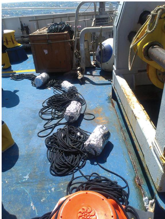
Figure 3 Deployment of passive sampler cages on the MPLS.
