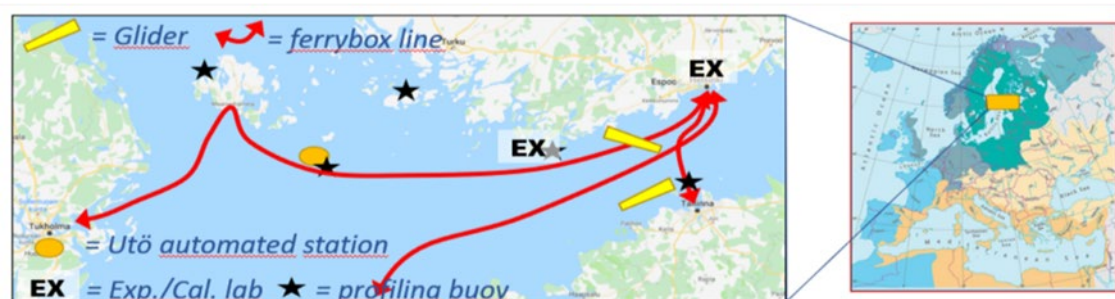
Figure 4. Map showing the key GoF PSS sustained platforms. Red lines represent FerryBox lines, stars are for profiling buoys, EX stands for experimental facility or calibration lab and the orange oval symbol is for Utö Atmospheric and Marine Station.
