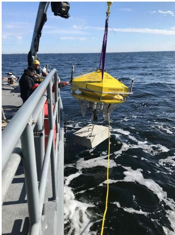
**Figure 7a.** The deployment of the Utö cabled profiler in April 2018; a crane is required because of the total weight of the system (800 Kg) and its height (4 m).
