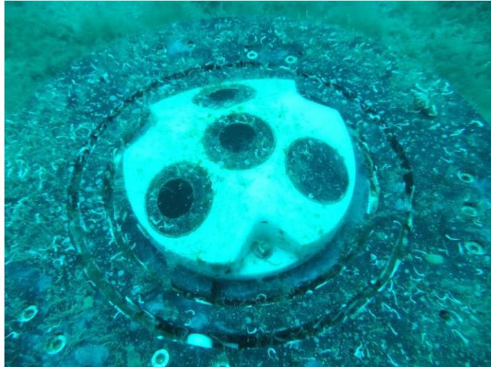
**Figure 14.** *New promising anti-fouling strips tested at the OBSEA Observatory, developed by Nitto Denko Corporation and commercialized by Nortek.*
