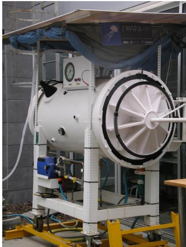
**Figure 16.** OBSEA's hyperbaric chamber for testing instruments before deployment.
