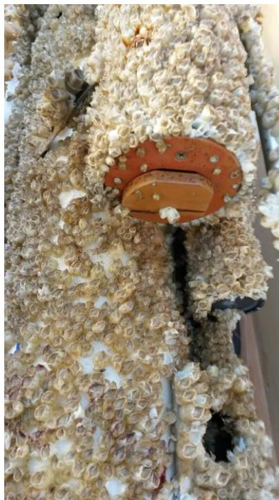
**Figure 13b.** *An example of biofouling on an instrument deployed at a depth of 5 m at Utö; a copper wiper is necessary to keep the optical window clean.*
