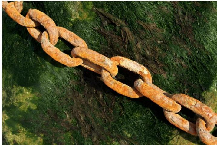
**Figure 15.** *Chains require periodic visual inspections to control corrosion.*
