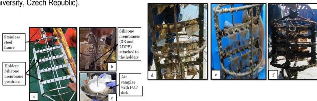
**Figure 6.2.9.2:** Passive sampling device assembly showing (a) the skeletal structure consisting of the stainless steel frame and holders; (b) the attached silicone rubber (SR) and LDPE membranes; (c) the air sampler with the PUF disk; (d) The mesh covered passive sampling devices recovered from POMOS; and (e-f) S1-GB experienced different degrees of biofouling.
