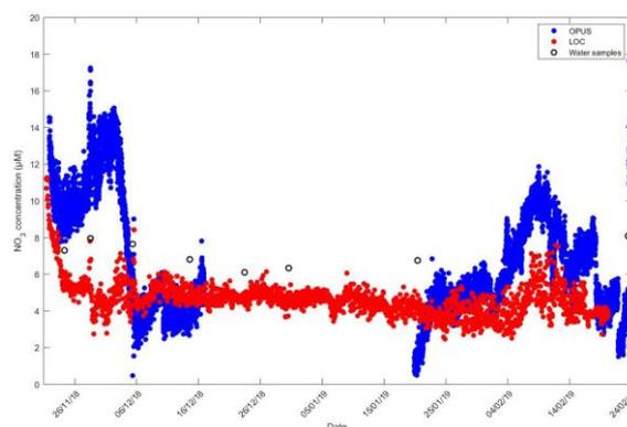
**Figure 6.3.5.1:** Nitrate measurements from the LOC (red) and Opus (blue) sensors for the first deployment period compared with water samples (black).
