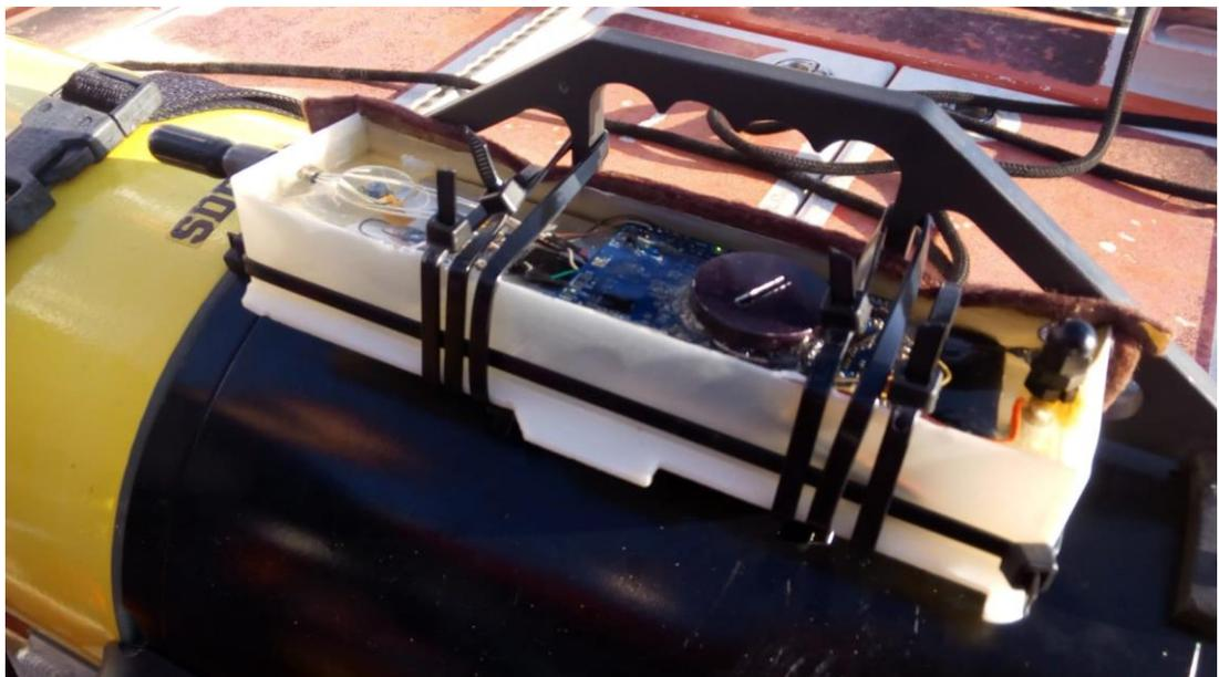
**Figure 6.3.1.2:** *The acoustic datalogger (BCB, Loggerhead Instrument) was turned on following the selected schedule and attached to the SOCIB glider SDEEP04.*
