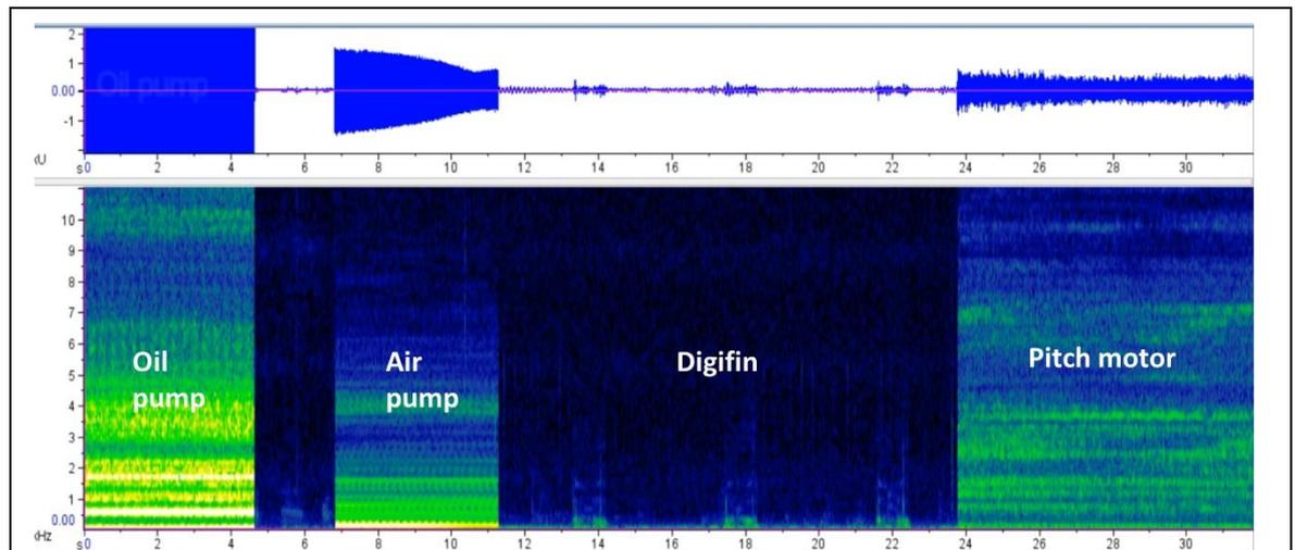
**Figure 6.3.1.1:** *Glider self-noise successfully recorded during the tests conducted as part of WP1. The time scale of x-axis is seconds. The original files were cut to show the different kinds of sounds. The testing experiment lasted longer.*
