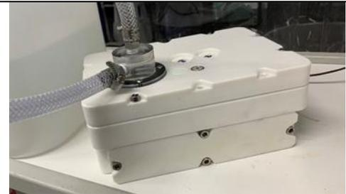
**Figure 6.2.5.1:** Integration of the ANB Sensors pH sensor into the flow loop system.
