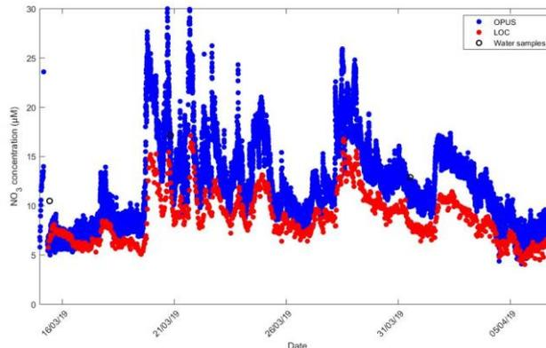
**Figure 6.3.5.2:** Nitrate measurements from the LOC (red) and Opus (blue) sensors during the FerryBox system deployment compared with water samples (black).
