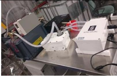
**Figure 6.2.5.3:** Integration of the ANB Sensors pH sensor, the AFT Sunburst pH sensor and the Contros pCO<sub>2</sub> into the flow loop system.
