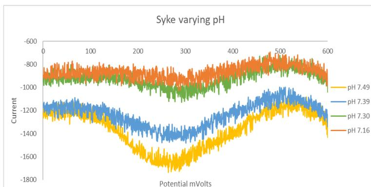
**Figure 6.2.5.2:** Current vs Potential plots for different pH waters, validated by the AFT-pH system.
