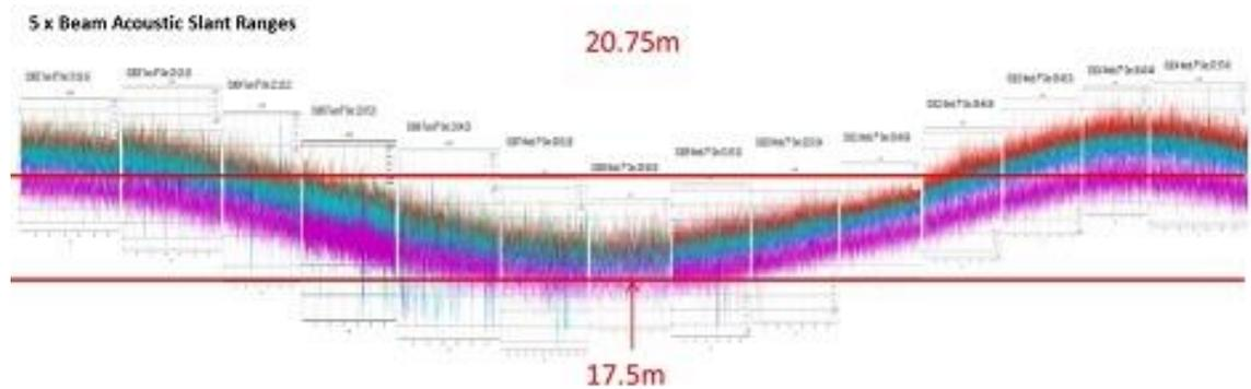
Taking a subset of this (1804), detailed comparison with the pressure sensor shows highest noise on the vertical beam, which is possibly attributable to signal saturation of acoustic return, while the tilted Janus beams, which are averaged and resolved to vertical shows the highest coherence with the pressure sensor. Note though that the pressure data is biased low at peak wave height due to spatial LPF action.
