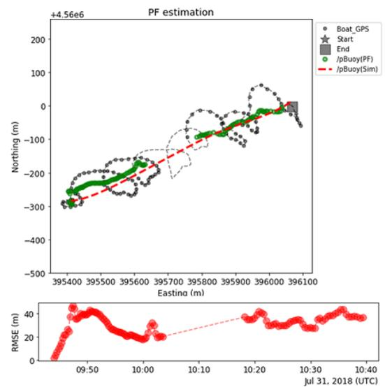
**Figure 6.2.1.4:** Moving target tracking: Test carried out to track a drifting buoy equipped with a modem. The x-y position of the observer (grey), the target (red), and the target's estimation (green) are represented on the top figure. The Root Mean Square Error (RMSE) is represented in the bottom figure.
