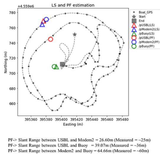
**Figure 6.2.1.3:** Static target localization: Test conducted to localize the modems deployed in the OBSEA, using LS (triangles) and PF (circles) algorithms, and their ranges from an observer (grey dots). The slant range obtained using PF and the ones measured with the modems are also represented (bottom).
