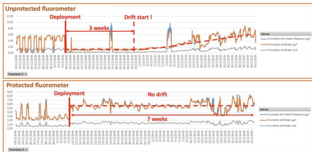
**Figure 6.2.11.2:** Fluorometers, 2 first months of deployment. Top: Unprotected fluorometer – Below: Protected fluorometer.
