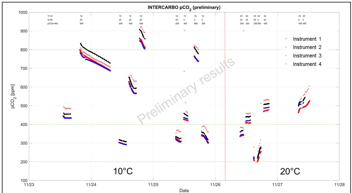
Figure 6.3.2.6: Comparison of four different pCO<sub>2</sub> instruments during the INTERCARBO experiments (preliminary result).
