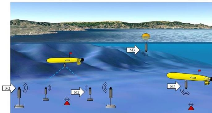
**Figure 6.2.1.1:** *Acoustic modem deployment scenario.*
