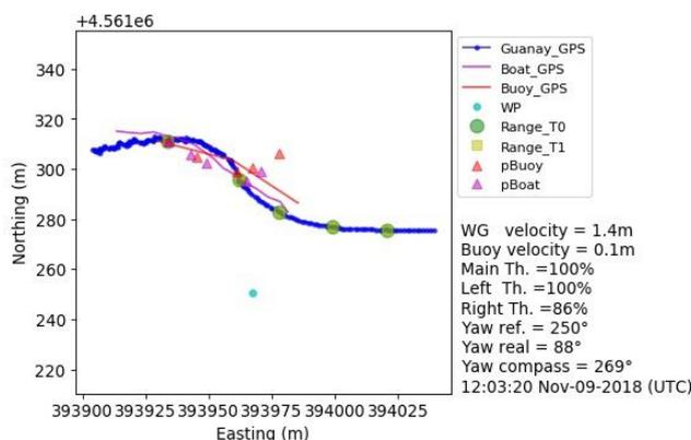
**Figure 6.2.1.5:** Moving multi target tracking: Test conducted to track a drifting buoy (red-triangles) and a boat (purple-triangles). Using an AUV (blue line).
