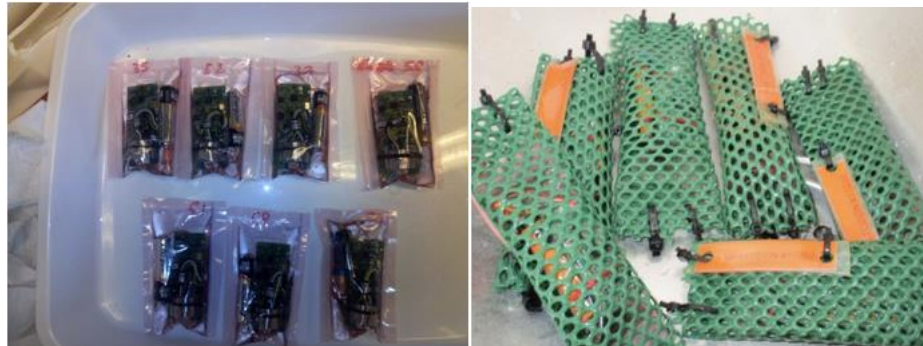
Figure 5: Left: electronic card packaged in heat-sealable bags. Right: T/P probes with protective grating.
