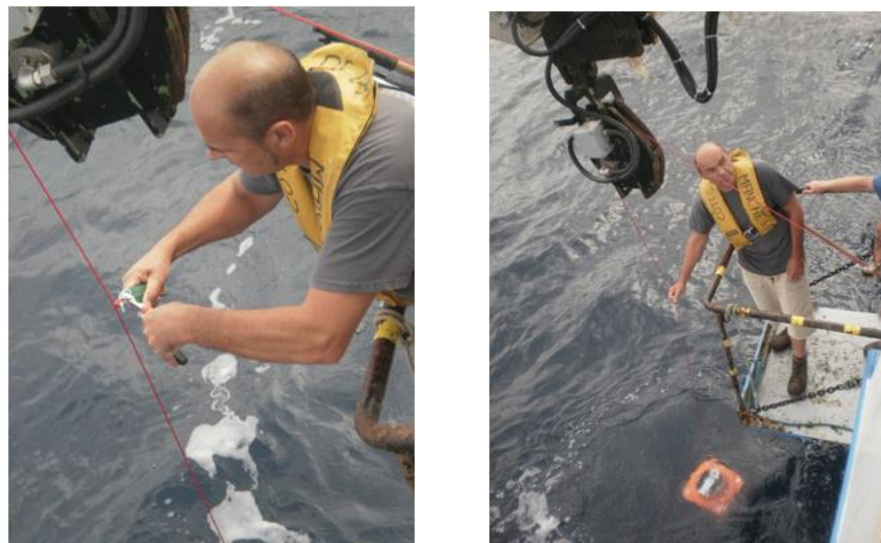
Figure 6: Left: temperature sensor in a Mastodon2D mooring line. Right: end of the recovery, the frame appears at the surface.
