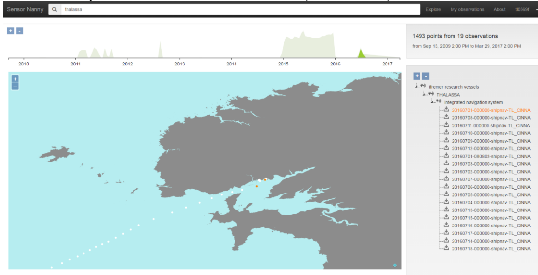
Figure 9: Thalassa research vessel navigation submitted in real time (every 5-minutes) through the owncloud client, as seen in the sensor nanny web portal
