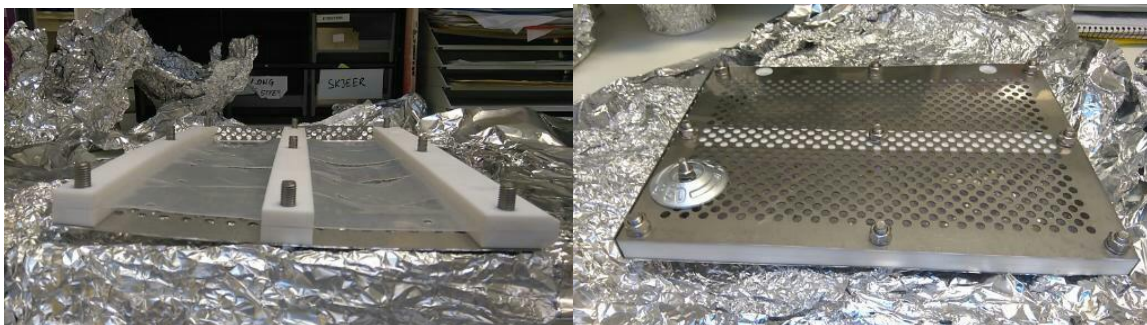
Figure 5.2: Left: Image of silicon passive samplers deployed in one of the new cages designed for Jerico infrastructures. Right; the cage ready for deployment.
