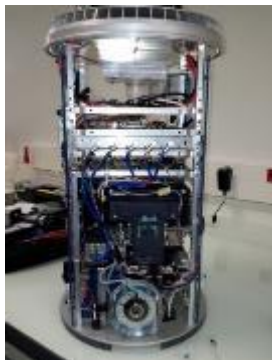
Figure 3.2: The CytoBuoy cytometer used in the Ferrybox system and the ferry boat line in the western Mediterranean.
