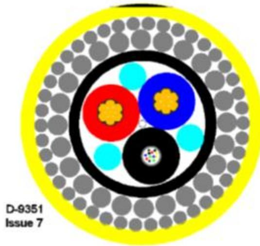
Figure 17. Section of the fiber and power cable.
