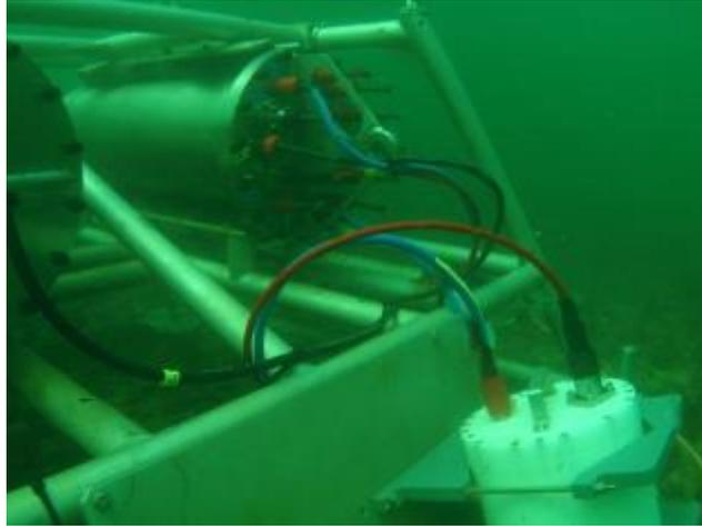
Figure 25. Connection between UNH node and instruments.
