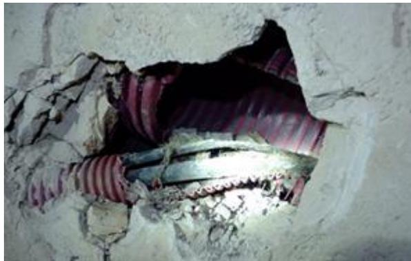
Figure 21. Destruction of optical fiber eaten by rats.
