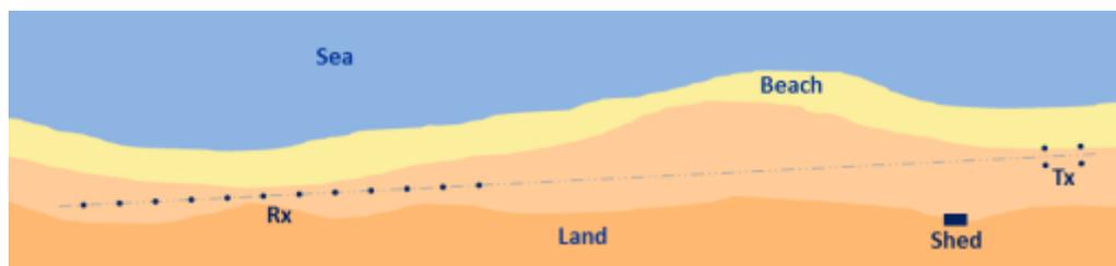
Figure 1. Typical setup of a phased array HF-radar system.
