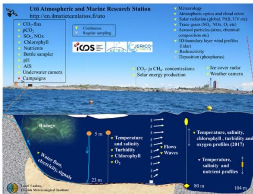
Figure 14. The Utö Atmospheric and Marine Research Station.
