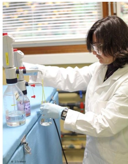
Fig. 4.4.2: Winkler sampling (with the courtesy of Ifremer).
