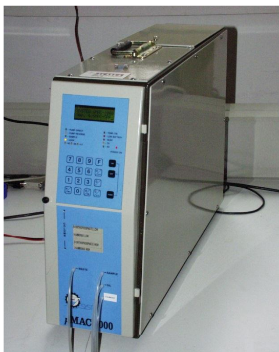
Fig. 4.3.1: Chemical sensor example: the Systea Micromac-1000.
