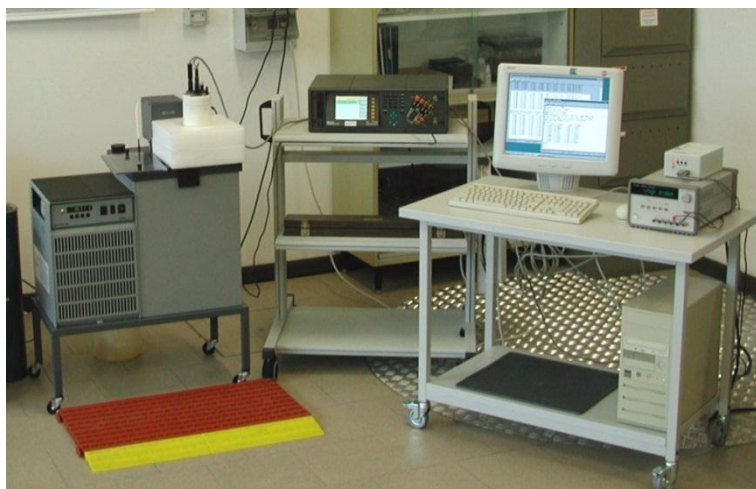
Figure 4.1.1: Testing of unit in thermostatic bath, controlled with reference system (left). Reference system for temperature using ITS-90 fixed points (right).
