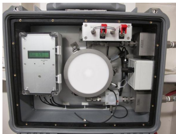
Figure 4.4.6. The NIVA-Franatech membrane based FerryBox pCO 2 system.
