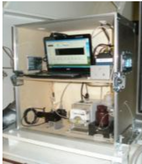
Figure 4.4.9. SMHI/Univ. of Gothenburg fluorescent pH-system on a setup onboard Transpaper.
