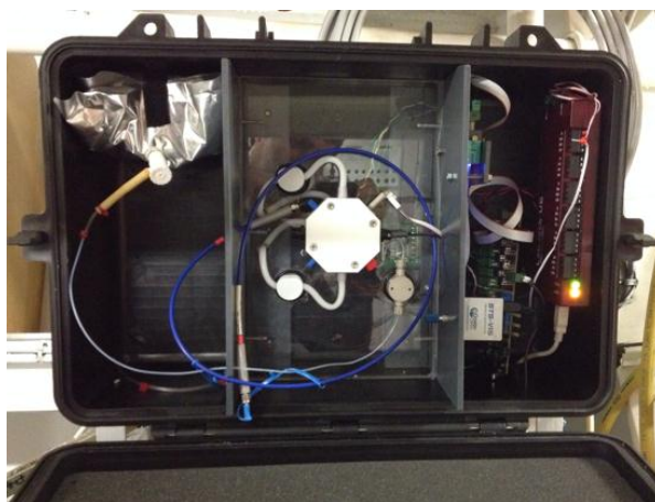
Figure 4.4.8. NIVA spectrophotometric pH-sensor mounted on MS Trollfjord.
