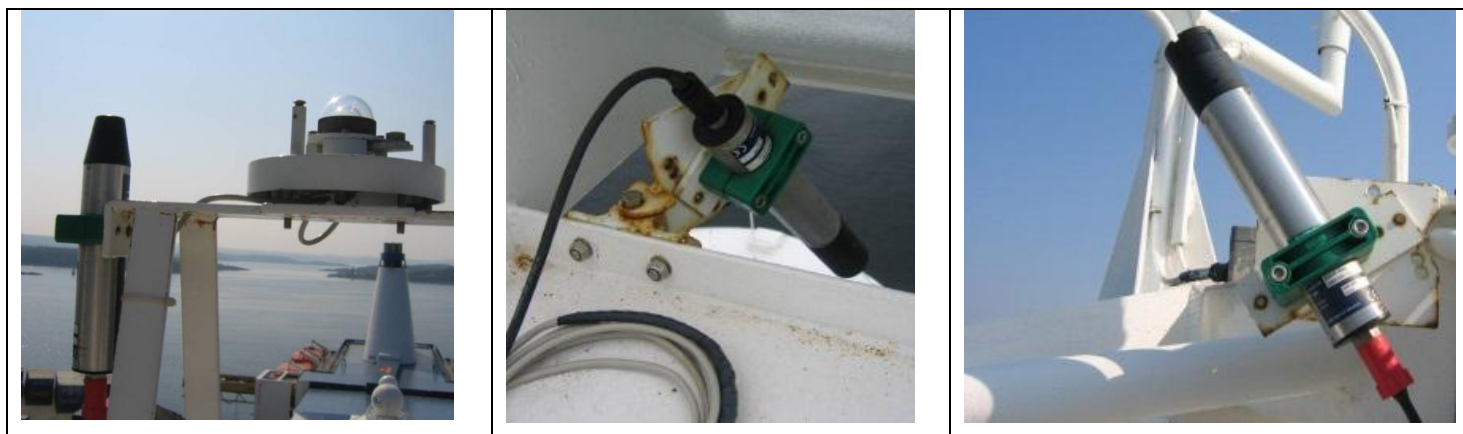
Figure 4.8.1. Installation on a ship of opportunity in Skagerrak. Radiance sensors can be mounted at different place on the ship.
