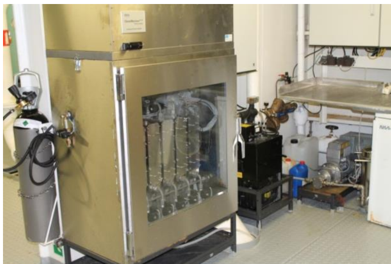
Figure 4.6.4. Chem Mariner installed at MS Color Fantasy (left) and one of the chamber opened to illustrate the membranes (right). By courtesy of NIVA.
