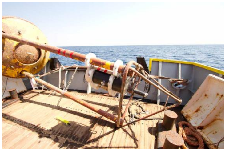
Figure 13: Sensorlab pCO 2 sensor, deployed on HCMR coastal buoy. By courtesy of HCMR.
