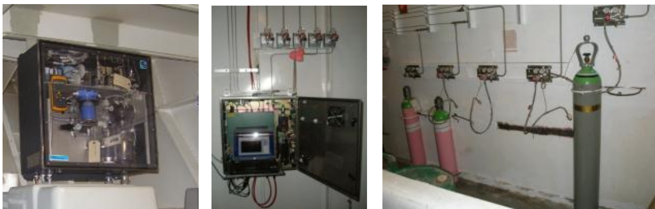
Figure 19 : CO 2 analyses system on ship TransPaper, left: wet box with analyses instrument, middle: dry box with computer and right: tubes with reference gases. By courtesy of SMHI.
