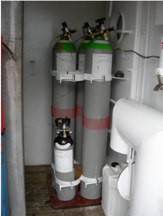
Figure 23 : Calibration gases installed in outside CTD garage on RV Cefas Endeavour.
