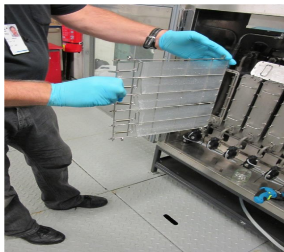
Figure 28 : Chem Mariner installed at MS Color Fantasy (left) and one of the chamber opened to illustrate the membranes (right). By courtesy of NIVA.
