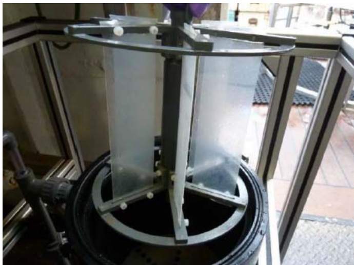
Figure 26 : Silicone rubber sheets mounted in a rack (by courtesy of CEFAS).
