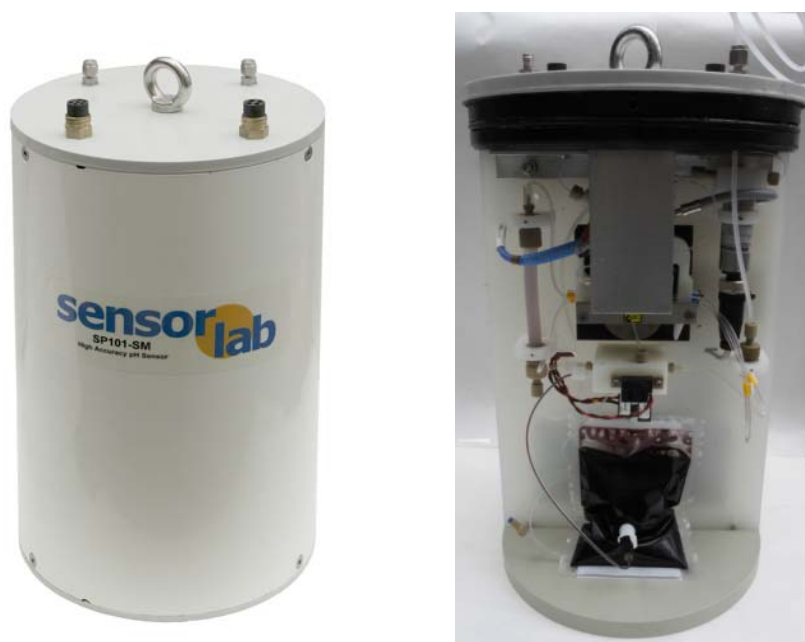
Figure 12: Sensorlab pCO 2 sensor. By courtesy of HCMR.
