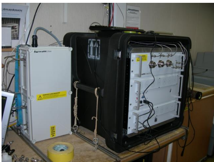
Figure 22 : Dry box installed in CTD annexe on RV Cefas Endeavour.
