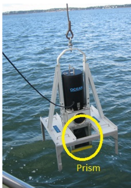
Figure 1 Light-framed version of sediment profile imager during sampling acquisition at the Arcachon Lagoon.
