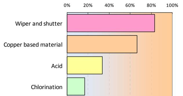
Shutters and wipers mostly protect sensors. Copper based material is also a technological solution. Acid cleaning and chlorination were also cited.
