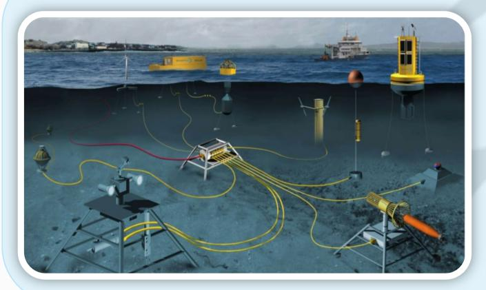
The Galway Bay Cabled Permanent Observatory (CPO) comprises a subsea platform cabled to shore, hosting a variety of scientific instruments for ocean observation and equipment testing and validation
