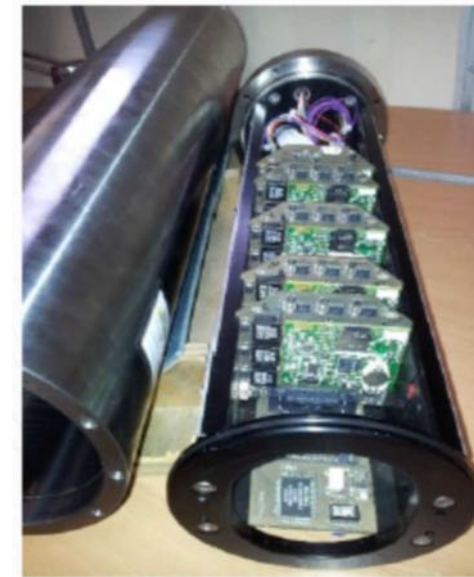
4000 m water depth version of the COSTOF2
