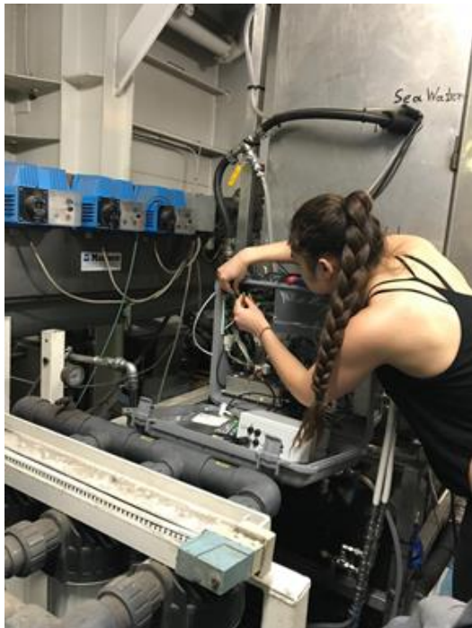
Fig. 1. Sabine Marty (NIVA) installing the pH sensor on H/S/F Festos Palace FerryBox on 27 March 2018.
