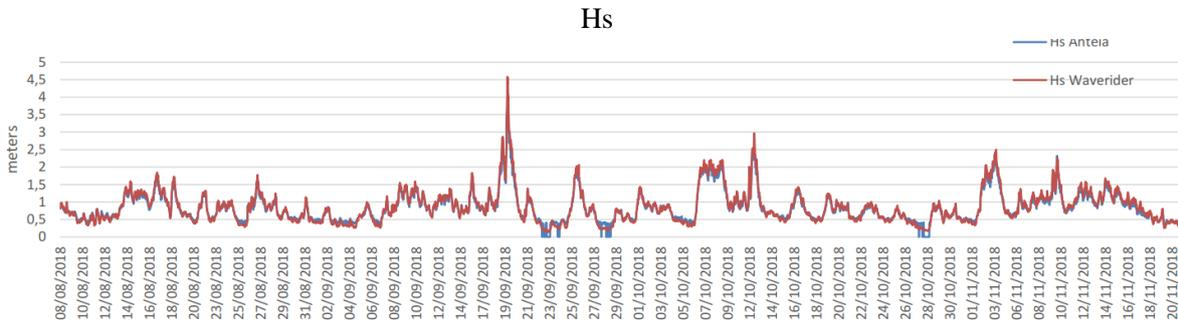
This plot shows Hs (time domain). There are some “0” values because ANTEIA buoy has a cut off filter tuned at 15cm, what means, that a wave below 15 cm is not considered as a wave.
