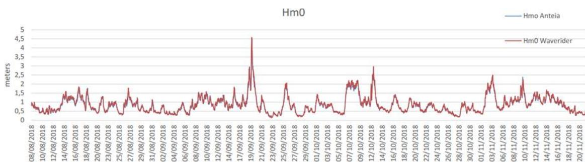
In this plot, Hm0 is shown. ANTEIA buoy has been working in different sea states between 0.5m and 4.5m of Hm0. With this different sea states, it has been possible to test the system in most relevant sea states.
