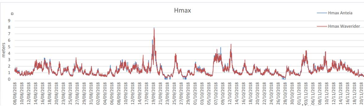
This plot shows a Hmax of 8m that was recorded during “Ali storm”. The correlation between both buoys reaches 92.84%.
